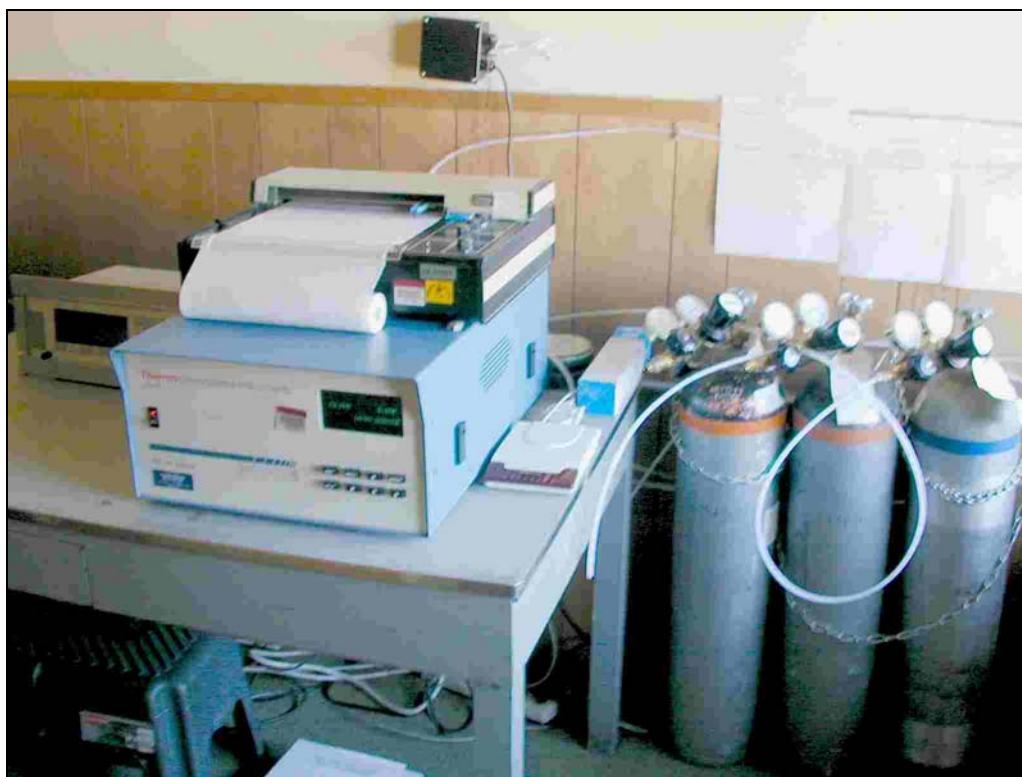
TECO 48 CO Analyzer with Strip Chart Recorder and Data Acquisition System Garden Monitoring Station
