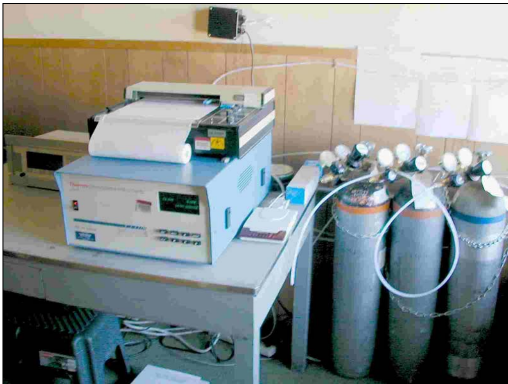
TECO 48 CO Analyzer with Strip Chart Recorder and Data Acquisition System Garden Monitoring Station
